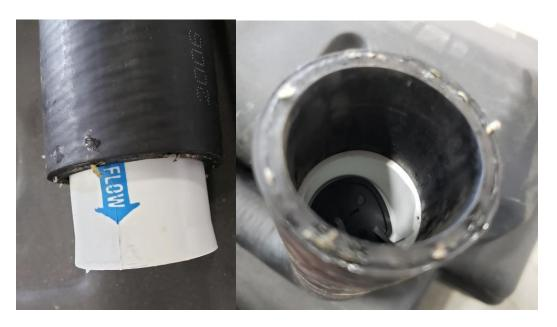
(Fig. 11) Insert 1-1/2" Fill Pipe ICV into fill hose with the "Flow" arrow pointing towards the fuel tank. This will need to be inserted deep enough to allow the fill hose to fit completely over the king nipple.
