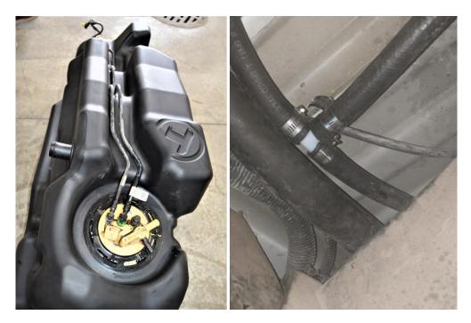
(Fig. 6) New TTITAN tank with fuel lines connected to the sending unit and in place.
