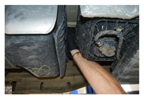
(Fig. 1) Disconnect fuel lines at the front of the OEM tank.
