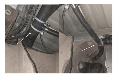
(Fig. 10) Zip tie the hose into place to prevent it from sagging in the future. Zip tie the tee to the top of the filler neck hose. Tighten all hose clamps appropriately.
